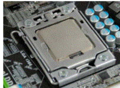
Align notches with notches on the CPU
