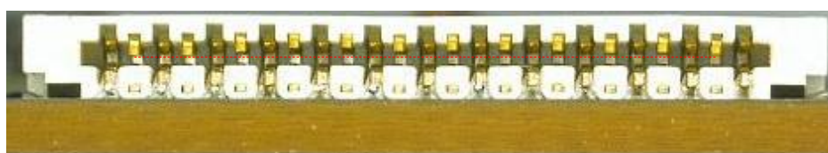
The upper contact point does not come down even if the cover housing is close.
