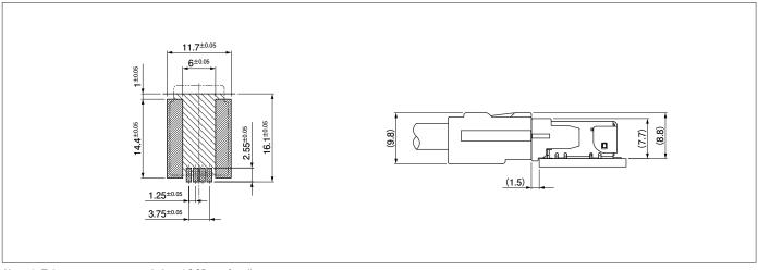
Note: 1. Tolerances are non-cumulative:  $\pm 0.05$  mm for all centers. 2. The dimentions above should serve as guideline. Contact JST for details.
