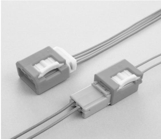
0.64 mm wire-to-wire and wire-to-unit connector with rigid design and spring lock mechanism. Spring force prevents incomplete mating during the mating process and keeps constant rigid connection between male and female connectors.
