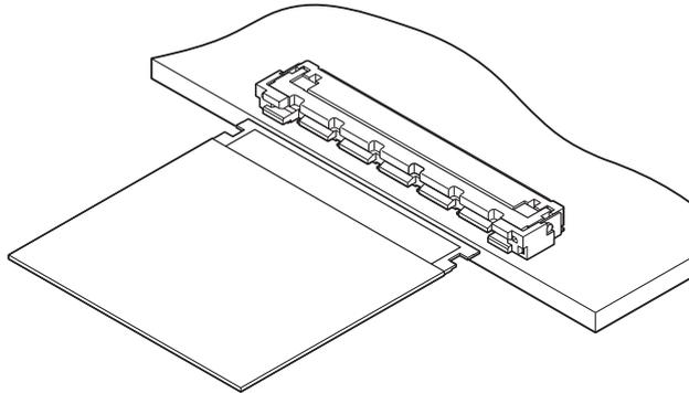
**This is 0.5 mm pitch connector for FPC which has the exclusive GND contact and enables high-speed transmission with connecting to the impedance controlled FPC. Adopting the auto lock mechanism that makes lock by performing the one action of snap-in-work, the workability improvement is realized.**
