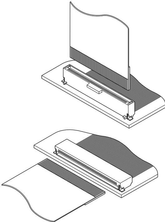
**0.5mm pitch non-ZIF snap-in type FFC connector.**
