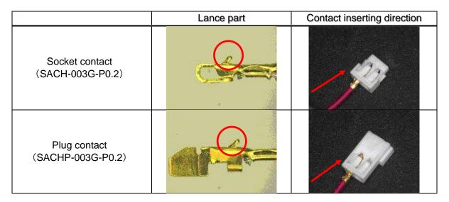
② Insert the contact into the housing without stopping to the innermost. When the contact is fully inserted into the housing, you can check that the insertion has completed with an audible clicking.
