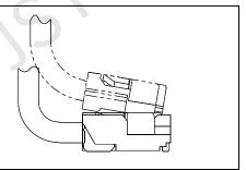
Unmate the connector by holding the wires at the angle within 15 degrees to the mating axis.
