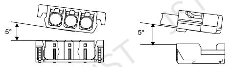
After mating the connectors, check secure mating, referring to the following points.
