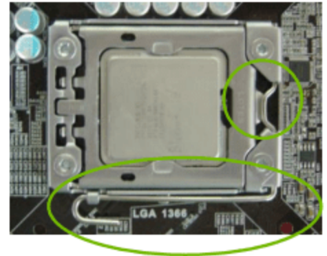
Align notches with notches on the CPU
