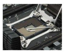
Note: After removing the CPU socket cover, it is recommended to store it in case you ever need to transport your motherboard. If you ever remove the CPU, it is highly recommended to reinstall the socket cover.
