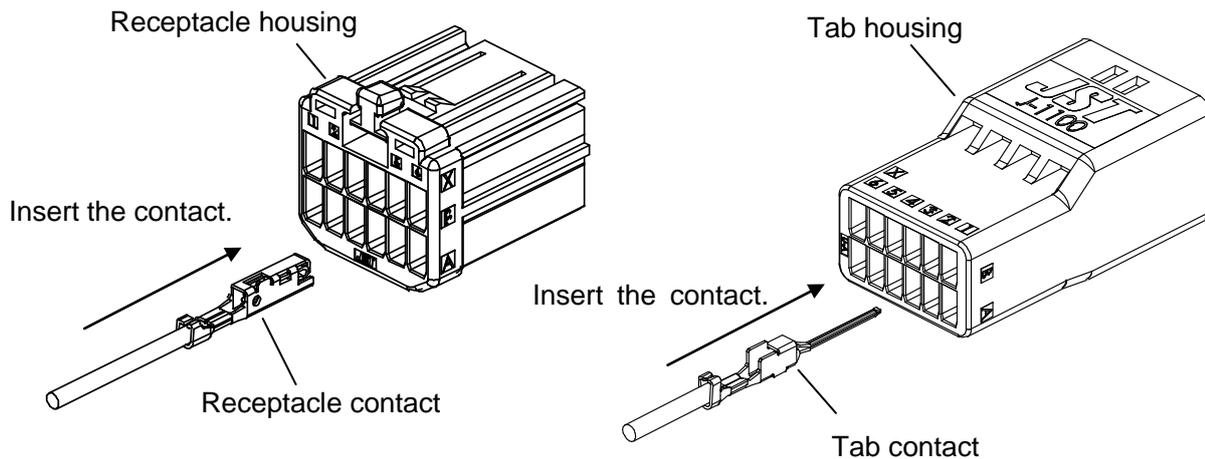
When the tab contact is inserted
