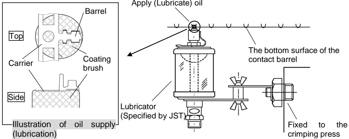
When the connector size makes applying oil difficult, we can provide oil lubricator for large-side contact. Contact JST if you would like.
