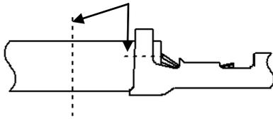
Remove the wire insulation.
