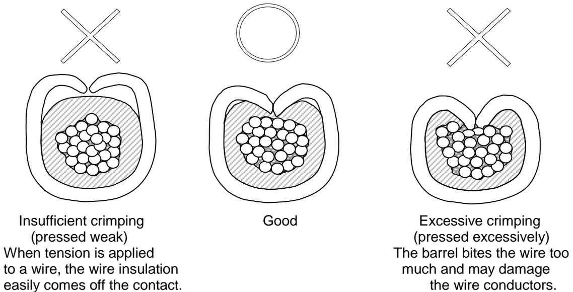
Check of the crimping condition at the wire insulation barrel
