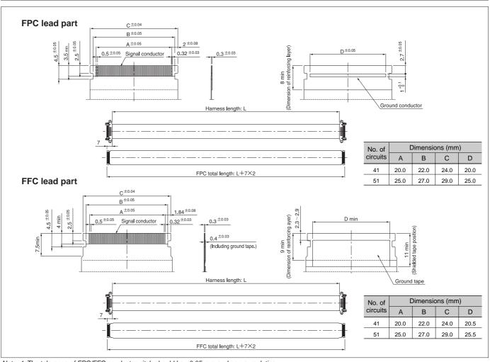
Note: 1. The tolerance of FPC/FFC conductor pitch should be  $\pm 0.05$  mm and non-cumulative.
