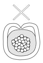
Insufficient crimping (pressed weak)
