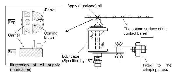
When the connector size makes applying oil difficult, we can provide oil lubricator for large-side contact. Contact JST if you would like.
