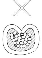
Excessive crimping (pressed excessively)
