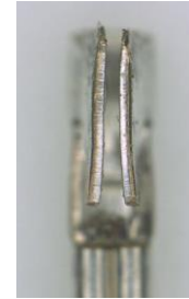
Too narrow mating part It may cause a collision with the mating header post.
