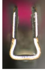
Too wide mating part Insufficient contact pressure may cause electrical discontinuity.
