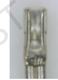
Too wide mating part Insufficient contact pressure may cause electrical discontinuity.
