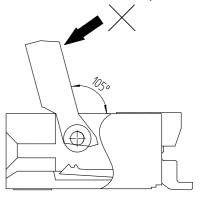
5. Please use two fingers when rotating the actuator as shown below. Otherwise, this may cause the actuator to malfunction.
