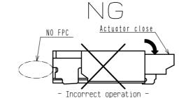
3. FPC insertion check (for using contacts on the top, for FPC pattern only applicable to FH34S\*)
