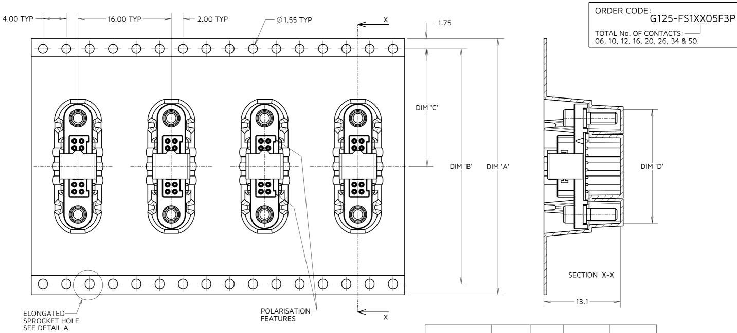
TAPE STRIP DETAILS ONLY. SEE SHEET 3 FOR CONNECTOR AND PCB LAYOUT DETAILS.
