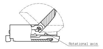
3. The actuator will not open more than 135°. Do not apply any force backward beyond this point. Otherwise, the actuator may come off or break.
