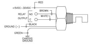
Figure 2 Typical wiring diagram for LL-01 series elements
