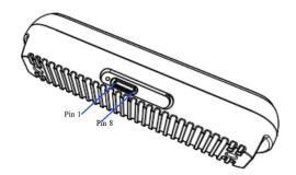
Gemini 335Lg Multi-device Synchronization Pin Placement.
