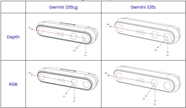
Table 4-5-2 Gemini 335Lg Coordinate System Schematic
