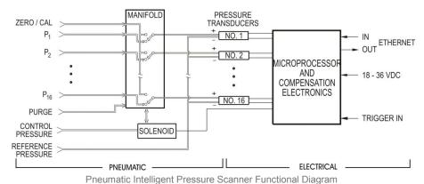
SENSOR SOLUTIONS /// NETSCANNER PRESSURE SCANNER 9216
